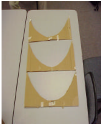
Parabolic ribs used in construction
